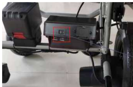
Main Power switch
