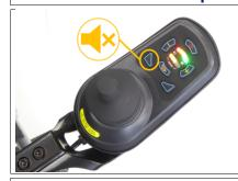
The handset controller has buttons to adjust speed and displays to indicate power remaining and speed setting.
