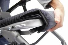
Unfold Power Chair by pushing the seat bottom down while pulling the release lever up.
