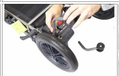
Install the anti-tip wheels. These simply press and lock into place.
