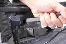
...insert the controller rod into the armrest fitting under the armrest...
