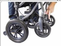
Check front wheels are positioned ahead to ensure smooth folding. Tip pull the chair backwards to align the wheels
