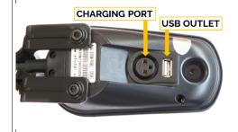
The charging port for your Power Chair is located under the handset for charging BOTH batteries simultaneously.
