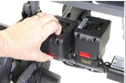
To remove batteries for travel or individual charging press the red tab upwards and slide the battery backwards.
