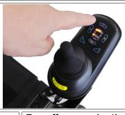
Turn off power using the POWER button on the hand controller..
