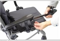
Slightly loosen the knurled knob, remove controller. Place controller and seat belt on seat pad. Retighten the knob to prevent loss.
