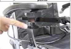
adjust the position of the controller and tighten with the knurled knob.
