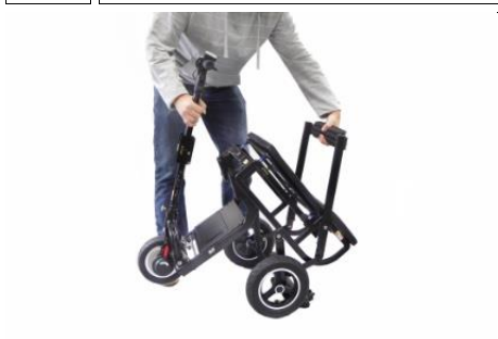
7 ...the scooter will unfold as you pull the seat back and steering column apart and ...
