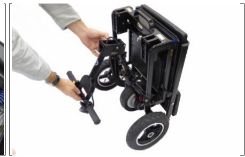
3 Pull the handlebars out and upward..
