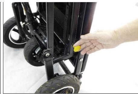
5 Locate small yellow stopper on side and pull to release front wheel assembly.
