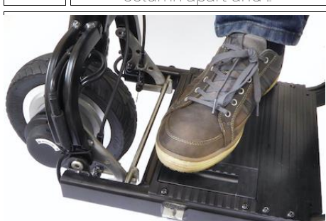
10 ...if not press your foot down onto the footplate to lock the scooter open.
