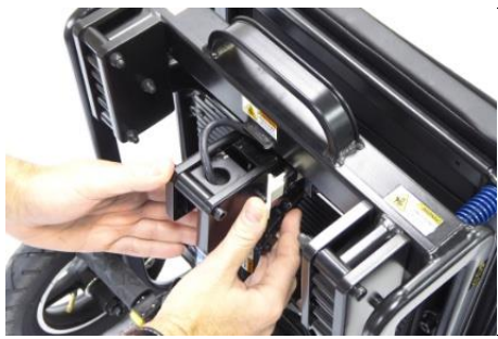
1 Release steering column latch...
