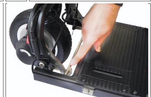
9 Make sure the locking latches have locked to the steel bar..
