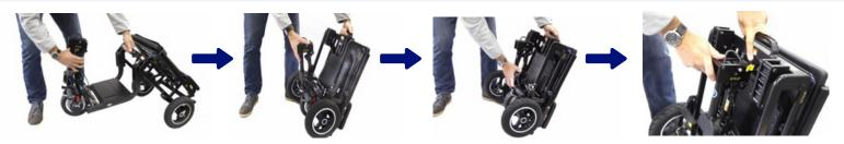
Grip the scooter by the steering column and carry handle & lift the seat frame to an upright position.
