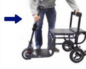
Hold the steering column and seat back, and pull them apart. The scooter will unfold and you will hear a click as it locks into its open position.
