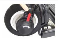
Check that the red magnetic brake lever is in the LOCKED position to engage the motor.
