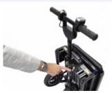
To turn the scooter into rolling luggage pull the handle bar up and press the yellow lever, securing it on the second stop point...
