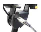
To charge, connect the power supply cable to the charging port located at the top of the steering column.
