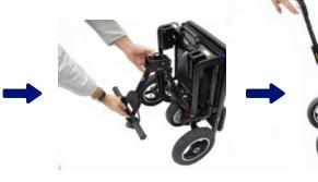
Push the yellow latch to release the steering column, allowing it to swing free.
