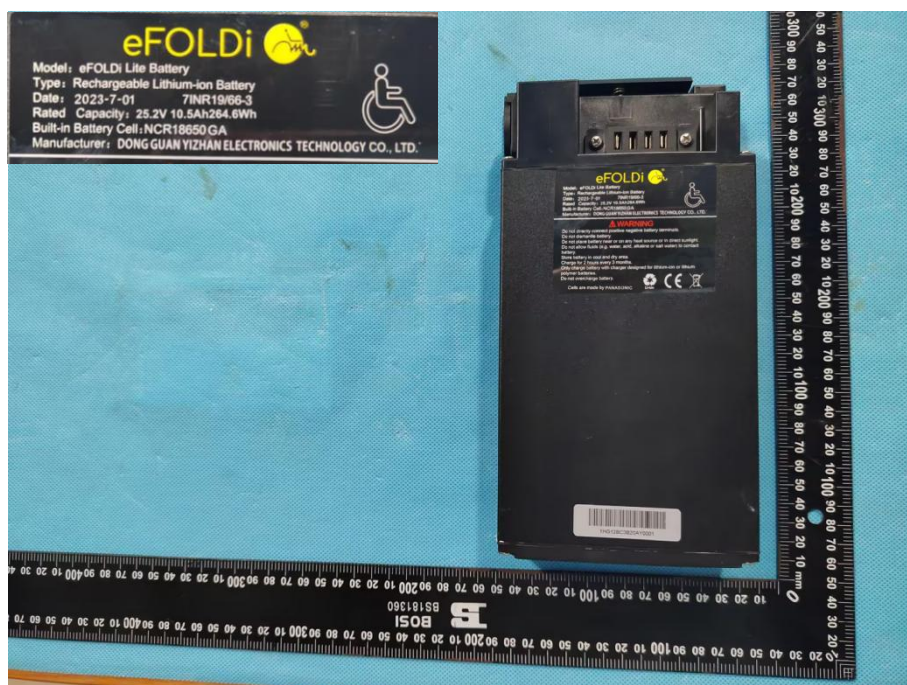
Photo 1 电池组正面 Front view of battery
