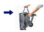
Press the steering column into the frame until latch "E" locks.
