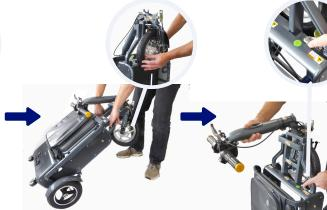
Lift the scooter to an upright position and lock the front wheel flat onto it's magnet in the frame. Locate latch "D" and press while supporting the steering column.
