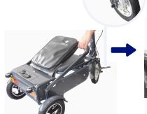
Fold the seat back down and the foot pegs into an upright position.
