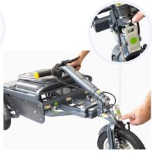
Press and release latch "A", folding the steering column flat against the seat.
