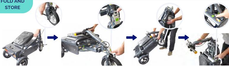
Fold the seat back down and the foot pegs into an upright position.
