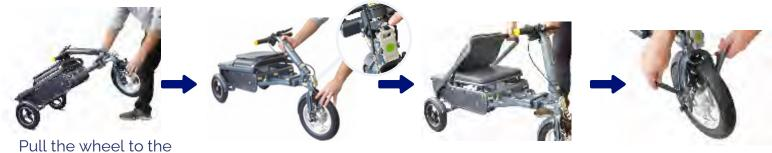
Pull the wheel to the front position and lower the scooter carefully to the ground.
