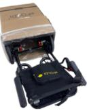
Stand the chair up and undo the seatbelt clip securing the chair in its folded position.
