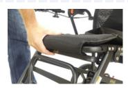
Press the folding lever (located under the front edge of the seat) & lift the seat to fold backwards.
