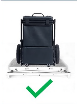
Lifter platform level and scooter-centred for balance.
