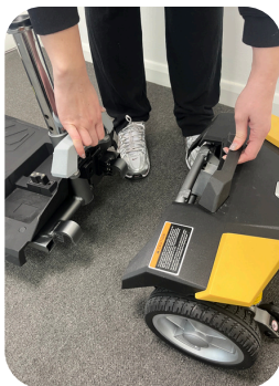
Lift grey handle to separate back section
