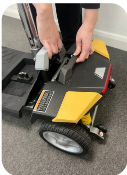
Lift grey handle to separate back section
