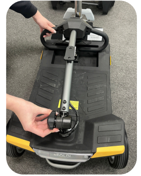
Turn the tiller cog to lower tiller until it is laying flat
