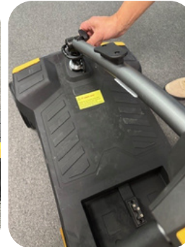
Turn the tiller cog to lower tiller until it is laying flat
